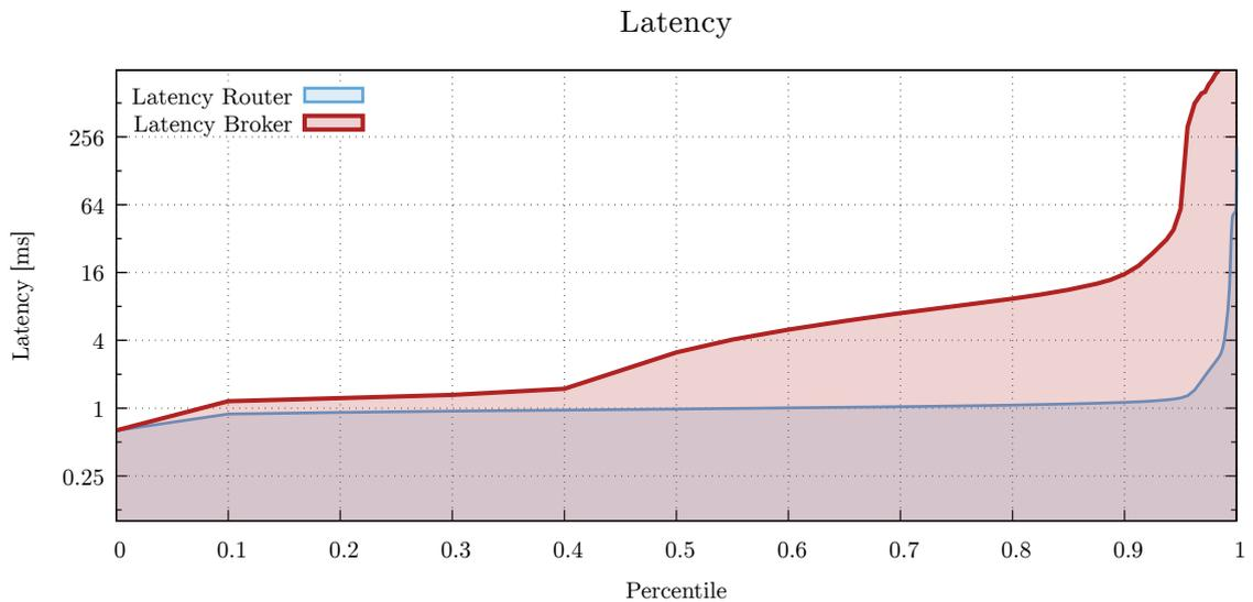
Figure 6.13: Latency comparison between topologies with only routers and with the middle-broker. The router network is here significantly faster.
